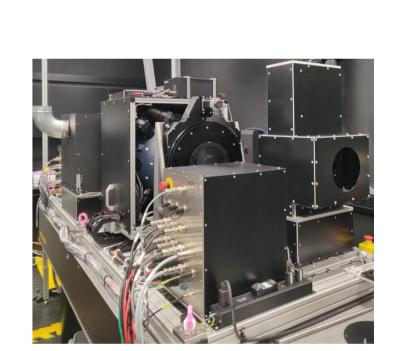
The STAR-CC-OGSE is a versatile facility for radiometric calibration and characterization (spectral response and straylight). It is provided with collimated beam source allowing monochromatic continuous fine-tuning from 260 nm to 2700 nm (narrow line-width <0.1 pm). The expected absolute calibration uncertainty is 0.5 %. It is now available at the NPL facility.
