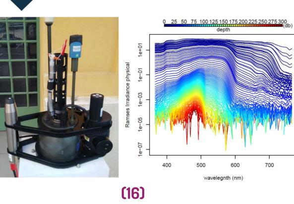
A Trios Ramses irradiance sensor has been integrated onto a Provor CTS5 (NKE) float and deployed for the first time at BOUSSOLE for testing. The next step will be integration of radiance/irradiance on the two-arms ProVal platform.
