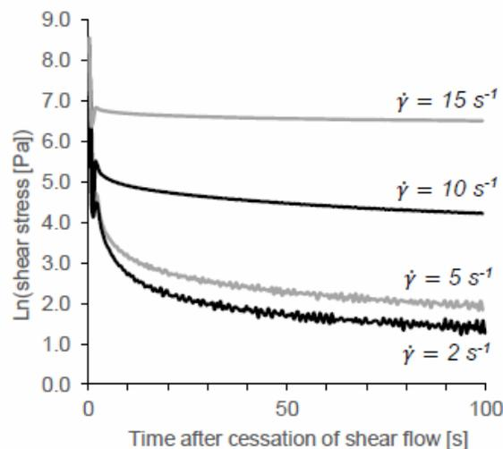
Figure 1: Stress relaxation observed following shear flow ( $\gamma = 100$ ) at the shear rates shown.
