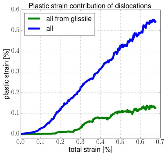
**Figure 1:** Plastic strain contribution from all dislocation resulting from glissile reactions (green) and total plastic strain produced by dislocations (blue) in tensile direction.
