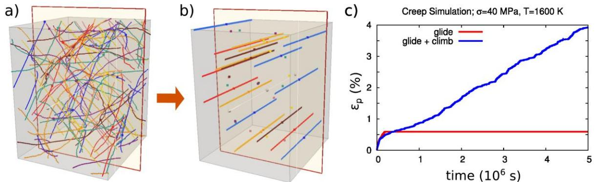
**Figure 1:** Sketch of full 3D- a) and 2.5D-DD simulation volume. c) Plastic deformation  $\epsilon_p$  vs. time, as obtained by 2.5D-DD simulations in creep conditions, assuming glide only (red curve) and glide coupled with climb (blue curve) dislocation motion.
