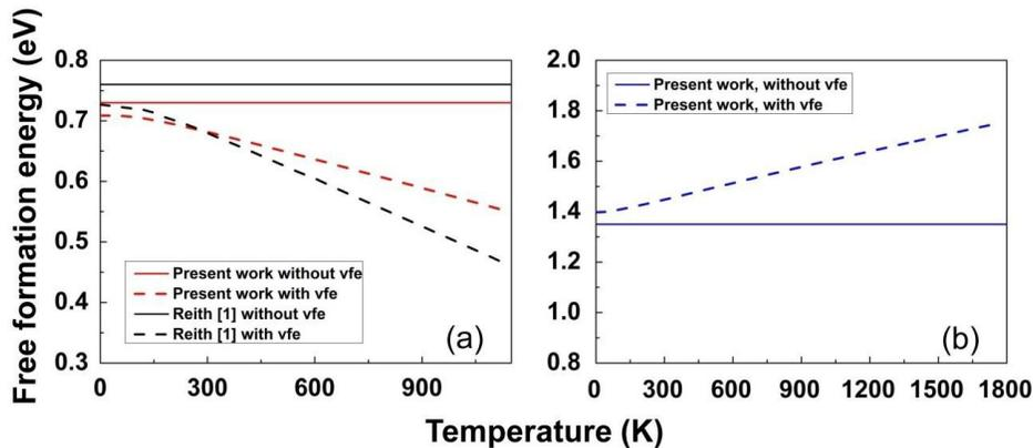
**Figure 1:** Total free formation energies of Cu (a) and O (b) in bcc Fe determined with and without considering the contribution of the vibrational free energy (vfe).
