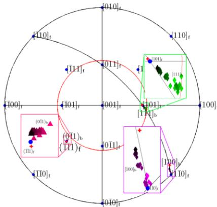
Figure 1. Stereographic projection of the simulated OR evolution.  $\Delta$  represents the projection of  $(0-11)_b$  plane, while  $\diamond$  shows the projection of  $[100]_b$  (purple) and  $[111]_b$  (green).  $+$  is the projection of values corresponding to the ideal O-line criterion. The darkness of the marker indicates the size of the precipitates, i.e., the darker is the marker, the bigger is the size.
