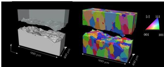
Figure 1. Reconstructions from X-ray tomography (left) and near-field HEDM (right).
