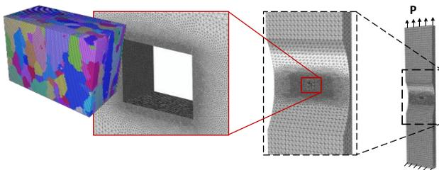
Figure 2. Concurrent multi-scale finite element model with polycrystalline region from experiment.
