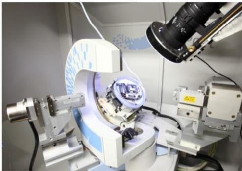
**Figure 1:** Assembly of the set up for the in-situ full-field measurements
