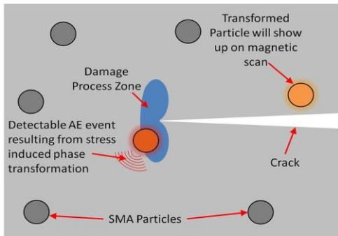
**Figure 1:** Embedded sensory particles, which undergo a detectable phase transformation in the presence of a crack.
