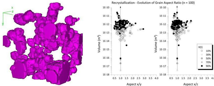
**Figure 1:** Visualization of the recrystallization front after 20% volume transformation (to the left) and statistics of grain volume and shape at advanced stages of growth (to the right).
