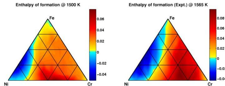
**Figure 1:** Enthalpies of formation (in eV) for the most stable crystal structures of Fe-Cr-Ni alloys computed using MC simulations at 1500 K (left). Experimental data from Ref. [1] are shown on the right.
