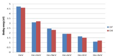
**Figure 1:** Comparison of predicted values of binding energies between He and various defects (HeV, Ne, Ar, Kr and Xe) with experimental measurements derived from thermal desorption spectrometry of bcc tungsten.
