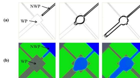
Figure 1: Dynamic drainage images: (a) experimental images of forced injection of non-wetting phase WP at 0.5ml/min (b) corresponding LBM simulations.
