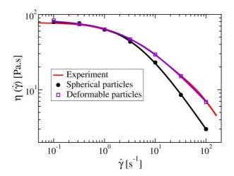
Demonstration of the recovery of the non-linear rheology of a polymer solution using the RaPiD deformable particle model.
