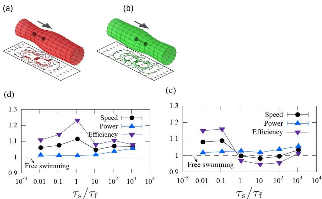
FIG. 1. (a) and (b) Numerical simulations of extensile and contractile dipolar swimmers in an elastic tube. (c) and (d) Effect of the interaction with the tube on the swimmer motility. The amplitude of the response in the swimmer speed and swimming efficiency depends on the ratio between swimmer and elastic timescales,  $\tau_s/\tau_f$
