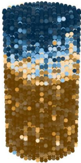
Figure 1 - a grain with dimensions 5nm in diameter and 10nm in height showing evidence of switching. The blue dots represent spins that have their original magnetisation whereas the gold dots represent spins that have reversed their direction.
