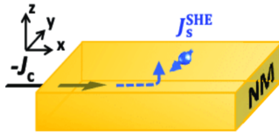
Figure 1: Spin Hall effect in a nonmagnetic material (NM), where J_c is the charge current and J_s^{SHE} is the spin current generated.[1]
