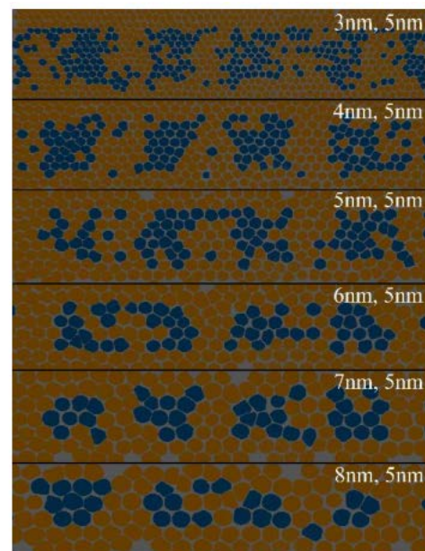
Figure 2 - HAMR simulations done on varying grain diameters (with height fixed at 5nm). The regions of blue and gold (blue representing spins pointing up and gold representing spins pointing down) are more distinct towards higher grain sizes, which is expected behaviour according to the magnetic recording quadrilemma.
