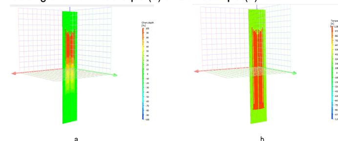
Figure 3. Conversion profiles for the Al/CuO thermite mixture at a pressure pulse of 3 GPa and time  $t = 30.5 \mu\text{s}$  (a) and  $t = 59.1 \mu\text{s}$  (b).
