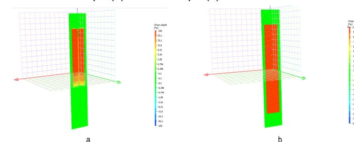
Figure 2. Conversion profiles for the Al/CuO thermite mixture at a pressure pulse of 4 GPa and time  $t = 24.8 \mu\text{s}$  (a) and  $t = 118 \mu\text{s}$  (b).
