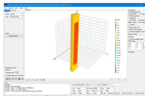
Figure 1. Computer configuration of the ampoule with the Al/CuO thermite mixture.
