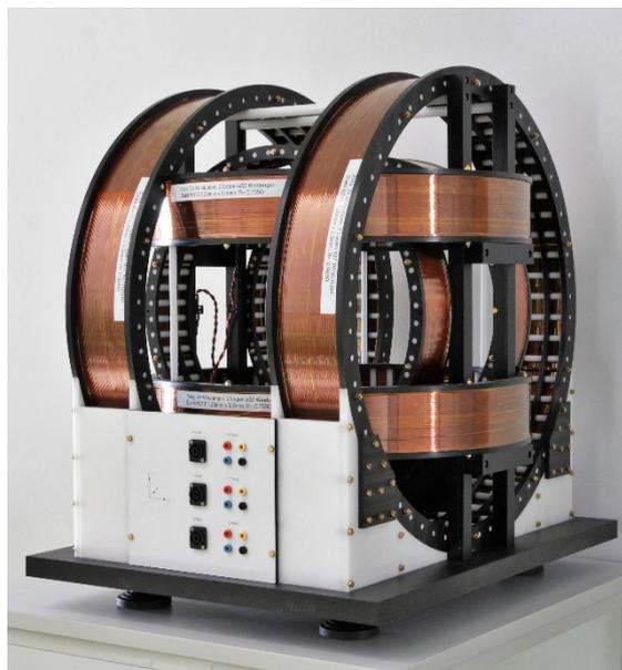
Figure 1: 3D Helmholtz coil developed for magnetic sensor calibration
