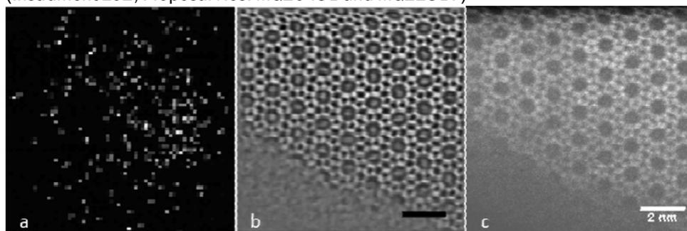
Figure 1. (a) A single detector frame from a high-speed direct electron detector (4D Canvas on a JEOL ARM200CF) demonstrating single-electron detection recorded at a dose of approximately  $4000 \text{ e}^-/\text{\AA}^2$ . (b) A ptychographic image of zeolite ZSM-5 and (c) the simultaneously recorded ADF image.
