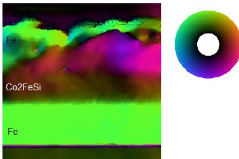
(DPC result from pixelated DPC measurement using the Medipix3 detector. The layer system made of Fe/Co<sub>2</sub>FeSi/Fe on MgO is visible, the deflection of the electron beam disc is shown color-coded by direction (color wheel on the right). The deflections are caused by magnetic contrast and diffraction contrast. In the upper Fe layer a domain wall can be seen.)
