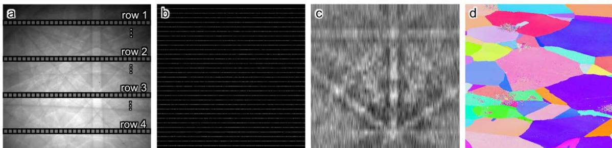
**Figure 1.** (a) Schematic of sparse sampling of an EBSD pattern. (b) Raw pattern acquired at 2200 frames per second, with 32 equally spaced kernel rows over the 2048×2048 pixels detector. (c) Post-processed pattern after background subtraction and inpainting. (d) Orientation mapping of a polycrystal Ni sample demonstrating the excellent indexing at the acquisition speed of 5150 points per second.
