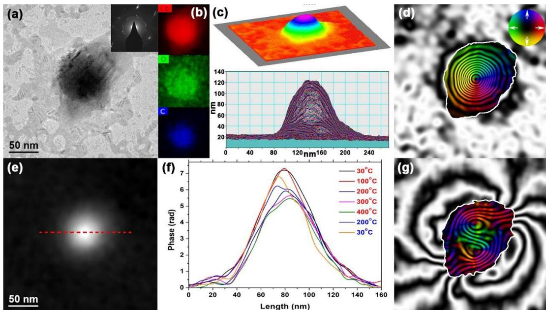
Figure 1. (a) TEM image; and (b) EDX chemical mapping of the annealed Co NP. (c) Morphology, thickness profile and (d) magnetic induction map of the Co NP. (e) Magnetic contribution to the phase and (f) line profiles of the vortex's thermoremanent behaviour. (g) S-shaped domain state at 300°C.
