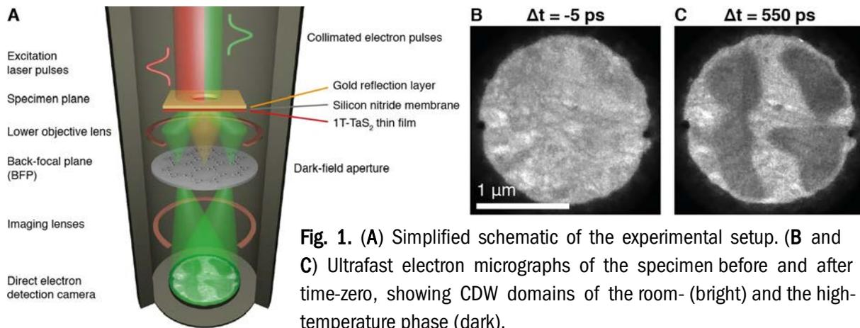
**Fig. 1.** (A) Simplified schematic of the experimental setup. (B and C) Ultrafast electron micrographs of the specimen before and after time-zero, showing CDW domains of the room- (bright) and the high-temperature phase (dark).
