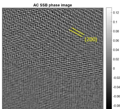
*Figure 1.* Ptychographic phase image of PEN crystallinity reveals conformational details. The structure between (200) planes are not observed in the images generated by the model that produced from XRD.
