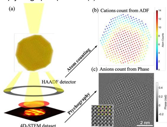
**Figure 1.** Schematic of quantitative electron ptychography applied to the measurement of local stoichiometry in ceria.
