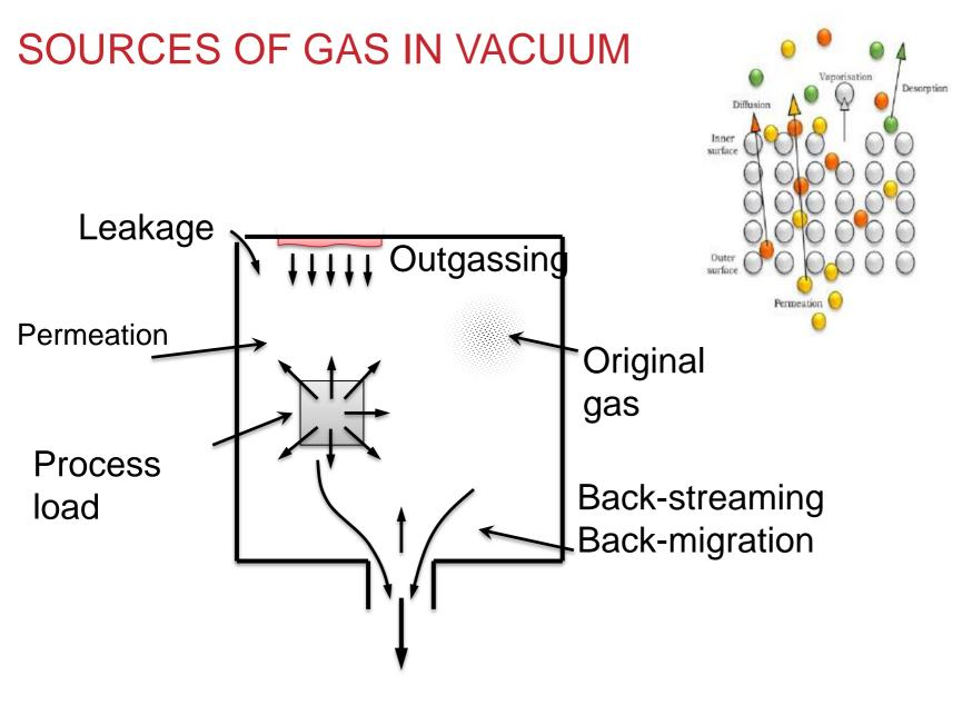
**Process Gas Load** is the gas added to the chamber from its process application: if present it is normally the dominant load;
